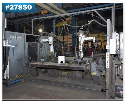
PANASONIC PRO SYS 2000 6-AXIS DUAL WELDING ROBOT TWIN MANIPULATOR CELL
