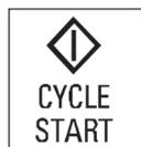
When a single cycle or the automatic cycle is Selected and the machine is waiting for "CYCLE START", it is possible to give the command also with the main teach pendant. If the selected cycle is the automatic one, the active override remains the one of the teach pendant; if the selected cycle is the single one, the active override becomes the one of the manual teach pendant.
