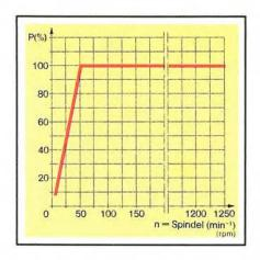
The available high power of the drive is transmitted through a three step motor, which is designed with a high torque rating, along the optimized ram to the cutting tool and is available for the whole length of the ram extension.
