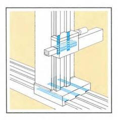
Reduction of idle times by quick positioning. High rates of acceleration and rapid traverse with low wear hydrostatic bearings in the X, Y and Z axes.
