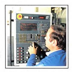
All Heavycut boring and milling machines can be operated in a conventional manual mode. It is further possible to operate in NC-assisted manual mode at any time.
