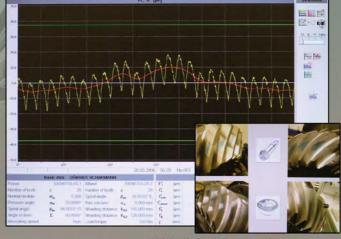
With digital photo option, captured images of realized contact patterns can be imported into the data file for the specific part-members
