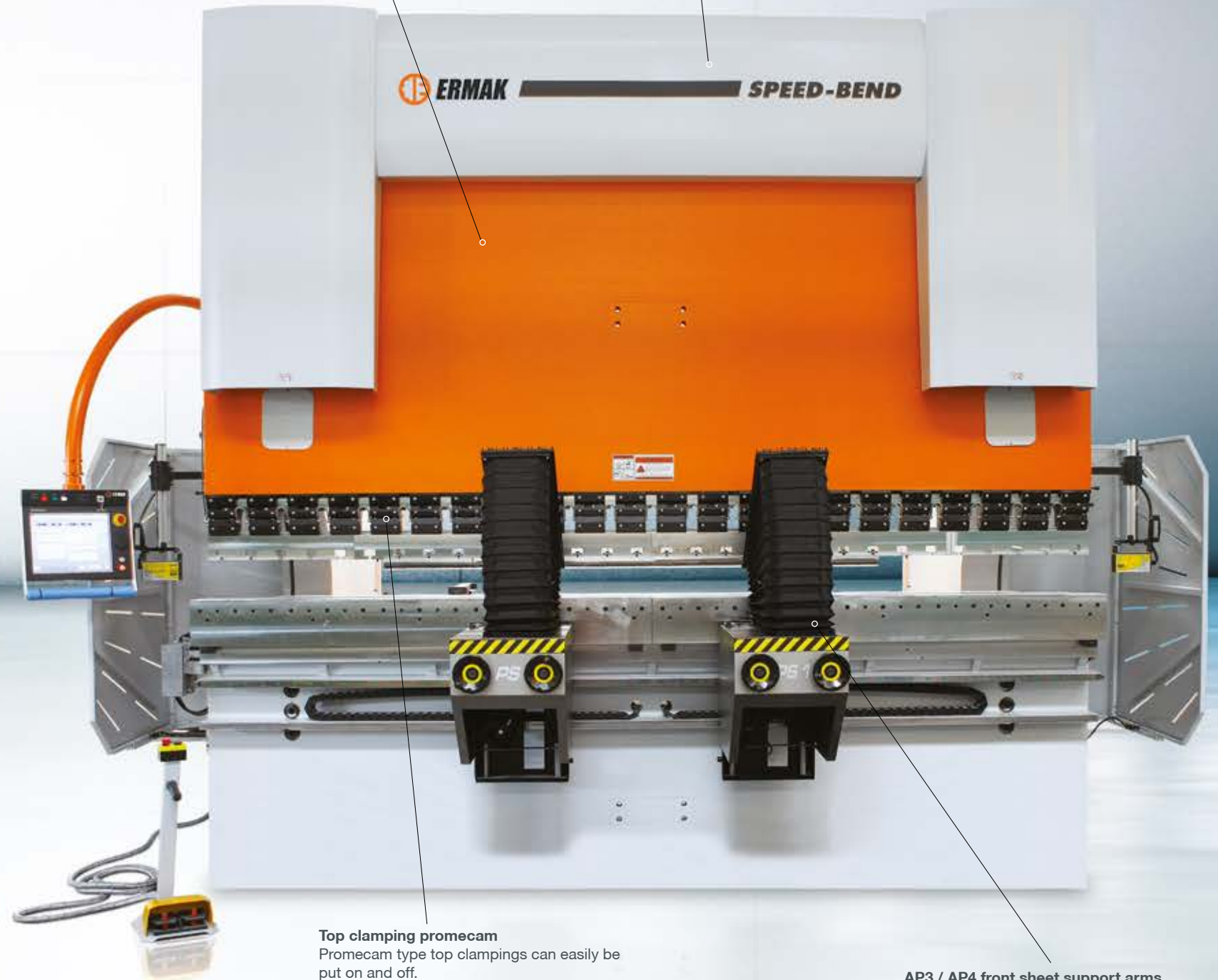
AP3 / AP4 front sheet support arms CNC controlled support arms prevents fast drop of heavy sheets after bending and is a great help for perfect bending.
