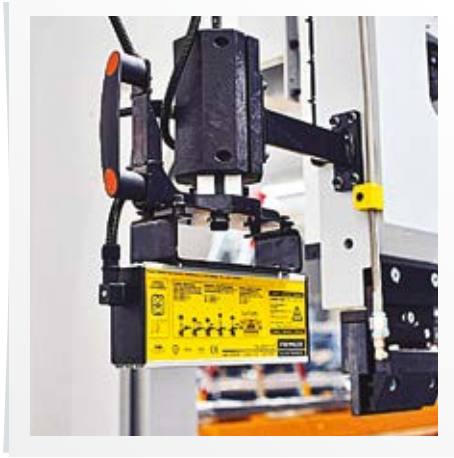
Fiessler Akas LCIM Protection System (S)
