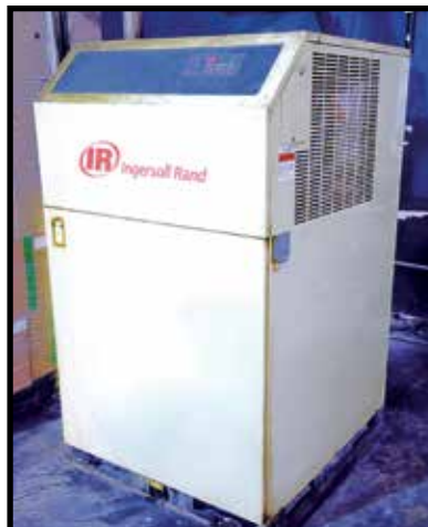
INGERSOLL RAND REFRIGERATED AIR DRYER
