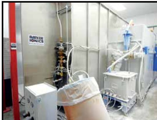
PARKER IONICS RECIRCULATING POWDER COAT BOOTH
