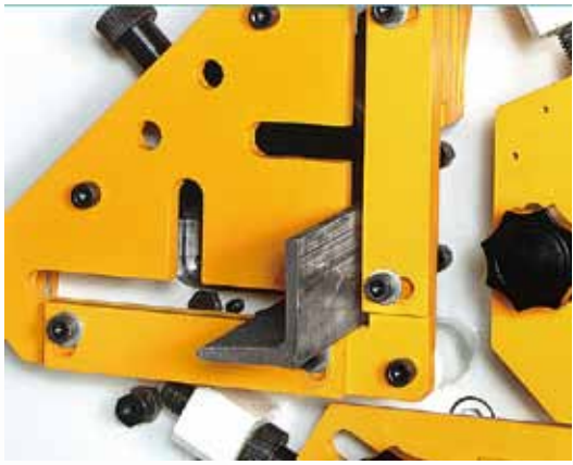
Angle Shearing Station
